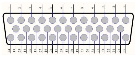
The connector model AMPSEAL-35P(P/n-1-776163-1) and the plug model (P/n-1-776164-1)
