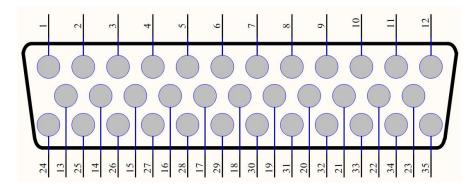
The connector model AMPSEAL-35P(P/n-1-776163-1) and the plug model (P/n-1-776164-1)
